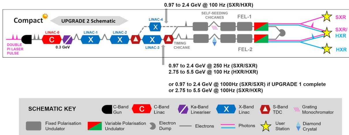
Figure 4.3.: CompactLight Upgrade 2 layout.
