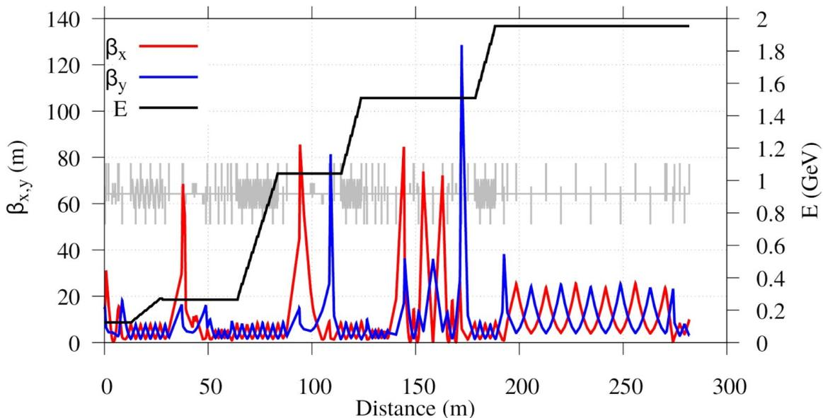
Figure 5.80.: Twiss functions and beam energy through Linac 4 to FEL-1 (**Option-iii a**)
