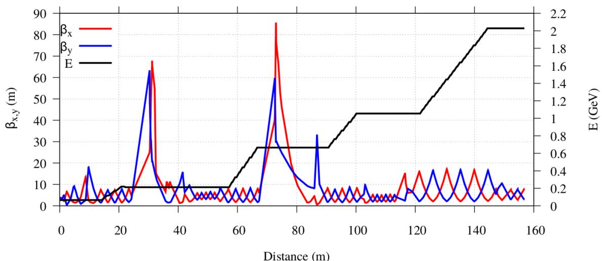
Figure 9.1.2.: Lattice  $\beta$ -functions and beam energy.
