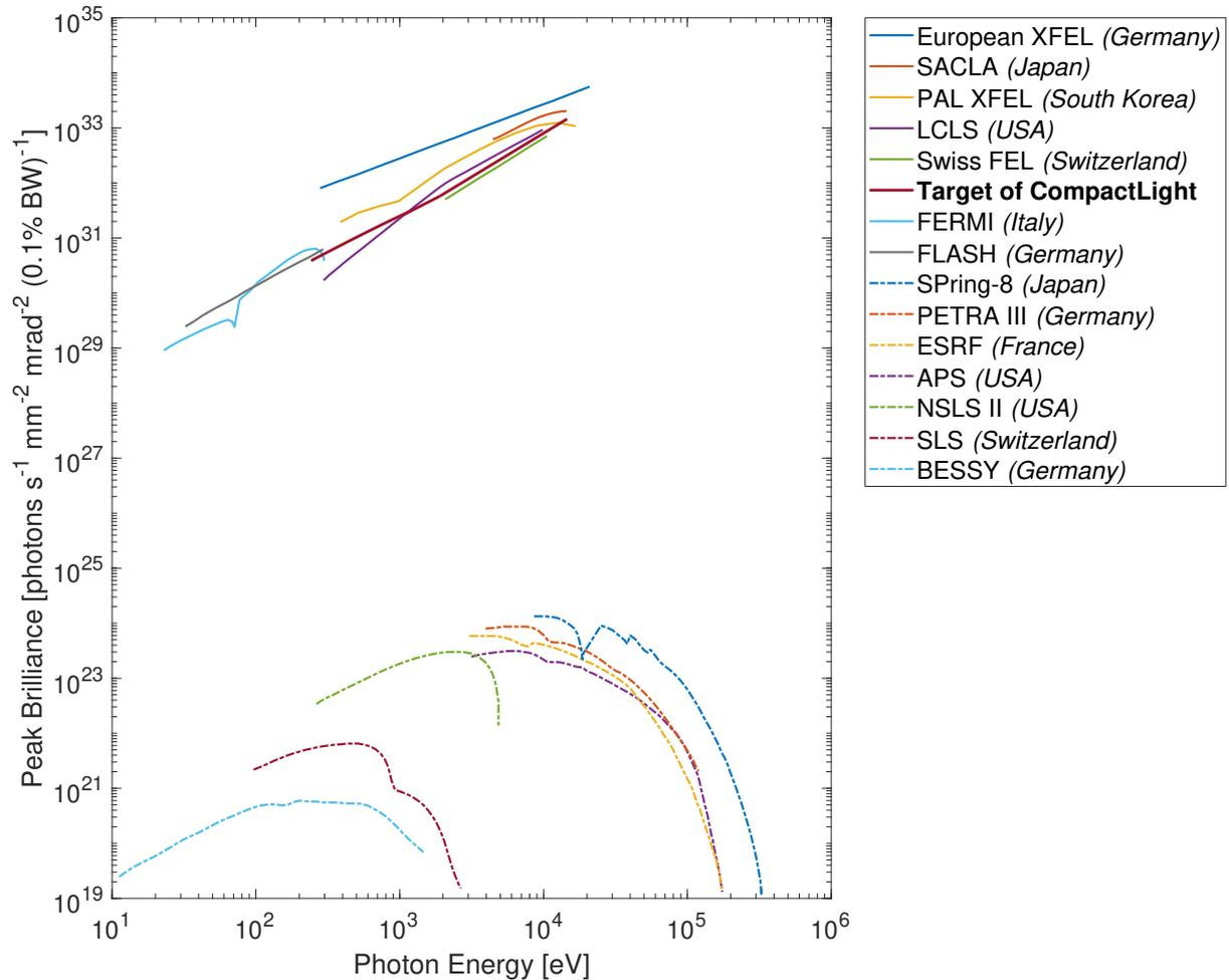
Figure 3.1.: Peak brightness as a function of photon energy for a selected set of x-ray sources. Free-electron laser facilities are shown in solid lines, and synchrotron facilities are shown in dashed lines. This figure is adapted from Figure 1 in [46].
