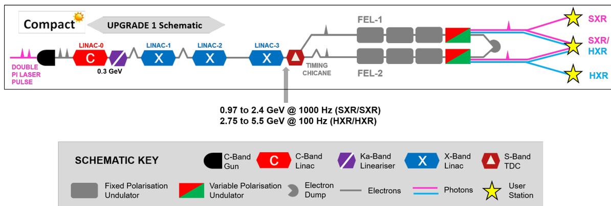
Figure 8.1.2.: Schematic layout of the CompactLight facility.
