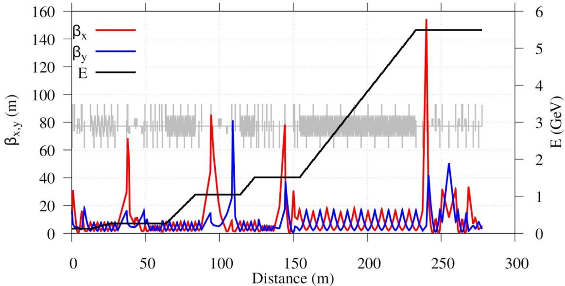
Figure 5.79.: Twiss functions and beam energy through Linac 3 to FEL-1 beamline (**Option-i a**)
