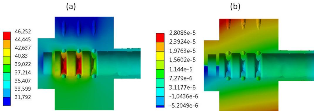
Figure 5.7.: (a) Gun temperature distribution and corresponding deformation (b)
