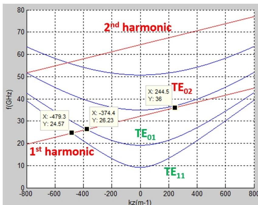
Figure 5.46.: Dispersion relation of the operating mode of the output cavity.
