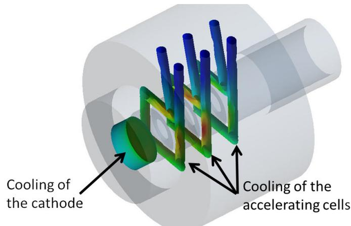
Figure 5.6.: Gun cooling system simulated in ANSYS.
