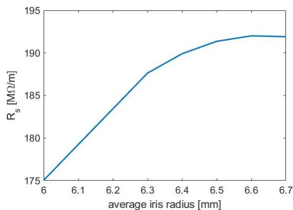
Figure 5.12.: Effective shunt impedance as a function of the average iris radius
