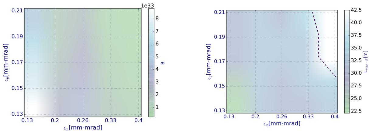
Figure 4.11.: Contour plots of FEL peak brightness (left hand side) and saturation length (right hand side) for the tracked bunch with artificially increased emittances. The dotted line on the right hand side plot corresponds to a saturation length of 36 m which is the undulator length specified in the design.
