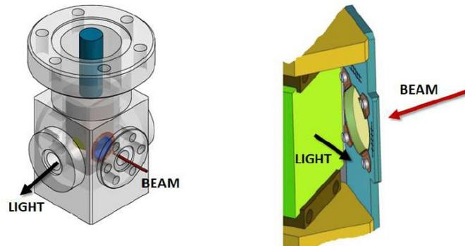
Figure 5.88.: Drawing of a compact view screen. A thin scintillator (typically  $100\ \mu\text{m}$ ) is placed normal to the beam direction. A 45 degree mirror on the back reflects the emitted radiation towards a detector outside the vacuum chamber.
