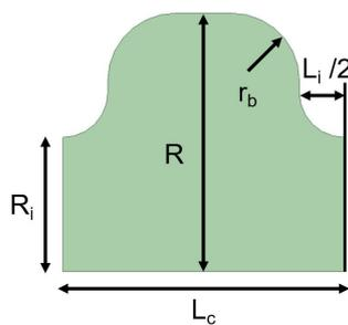
Figure 5.64.: Geometry of the standing-wave structure cell.
