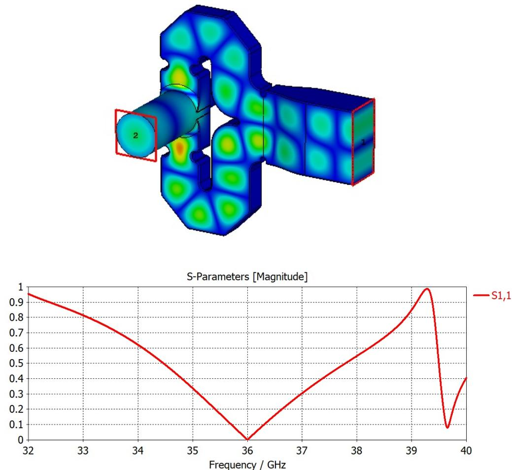
Figure 5.61.: TE20 to TE01 mode converter (top) and its matched S<sub>11</sub> parameters (bottom).
