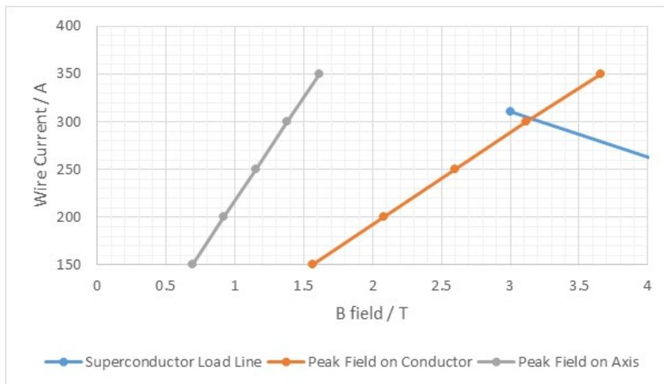
Figure 6.16.: Load line for chosen wire stack arrangement.
