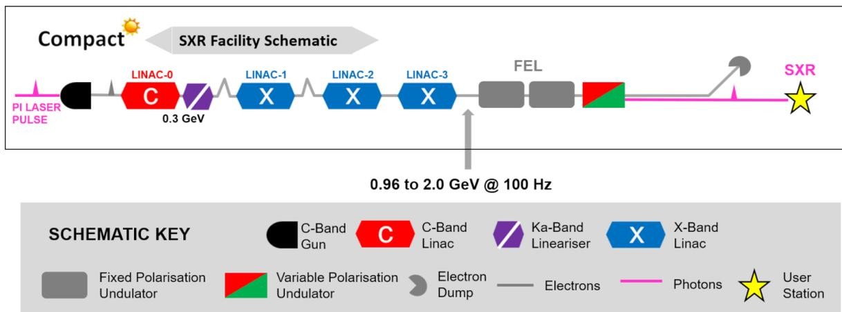
Figure 9.1.1.: Schematic layout of the SXR facility
