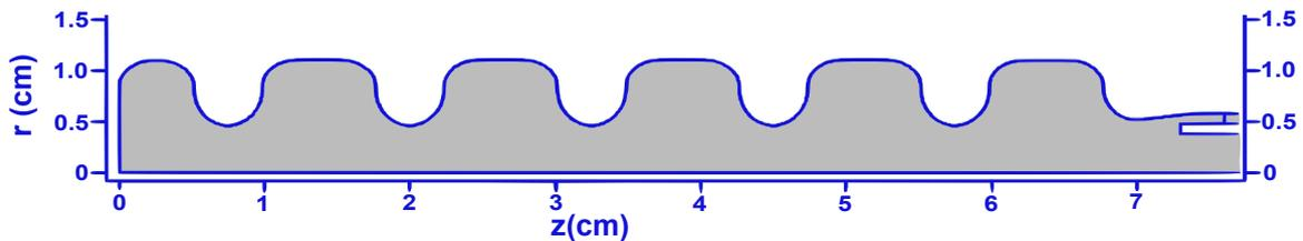
Figure 10.1.6.: Scheme of the longitudinal section of the 5.6 cell RF photoinjector with the coaxial coupler. The structure has symmetry of revolution around the  $z$  axis.
