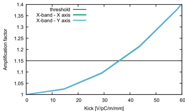
Figure 5.84.: Action amplification factor as a function of the amplitude of the transverse long-range wakefield kick at the 2<sup>nd</sup> bunch.
