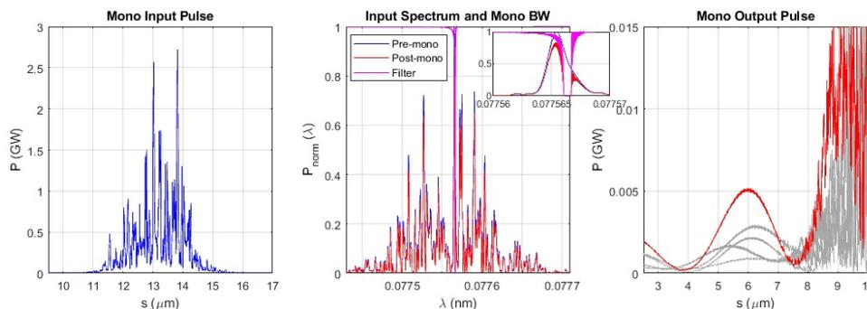
Figure 4.21.: Monochromator input pulse power profile (left), spectrum and monochromator bandwidth (centre, with zoomed horizontal axis in the inset) and output pulse (right). In the right plot only are shown results for four other shot noise realisations.
