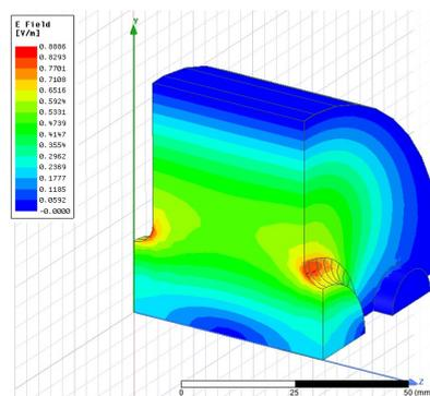
Figure 5.37.: The electrical field of single cell of standing-wave transverse deflecting structure.
