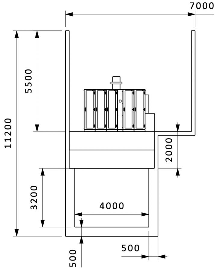
Figure 7.3.1.: Draft 5.0 XLS Tunnel and Infrastructure Hall cross-section (1:100)
