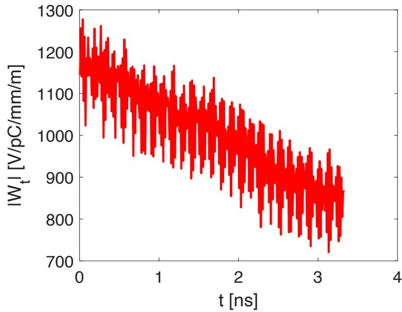
Figure 5.63.: Magnitude of the long-range transverse wakefield on a 30 cm TWS for a single XLS nominal electron bunch.
