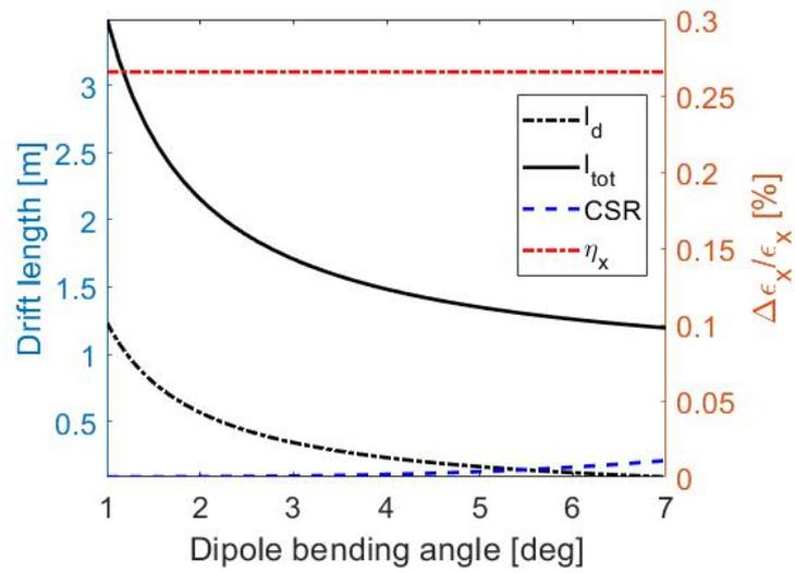
Figure 5.16.: Outer drift and total chicane length (left axis) and horizontal emittance growth induced by horizontal dispersion and CSR (right axis) vs. dipole bending angle, for fixed  $R_{52} = 23$  mm.
