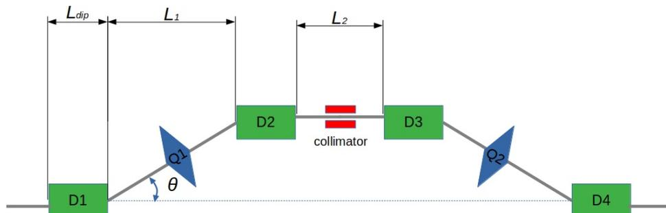
Figure 5.68.: A schematic of the bunch compressors
