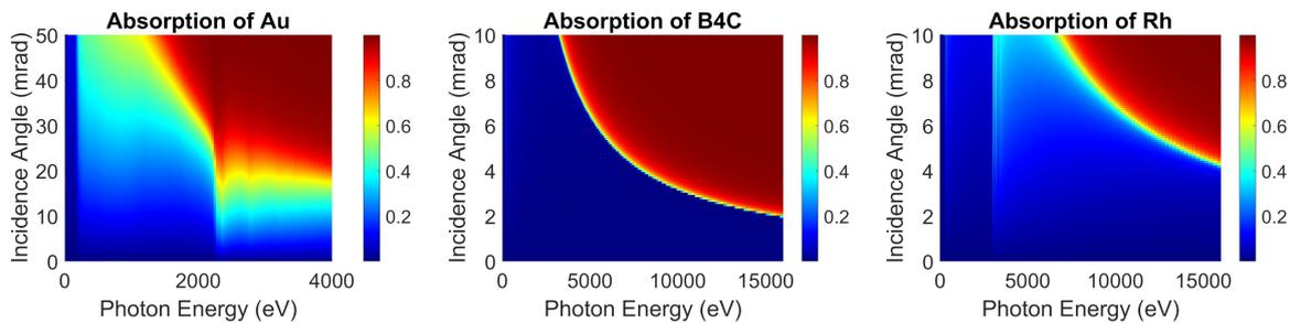
Figure 6.56.: Absorption of materials vs photon energy and incidence angle.
