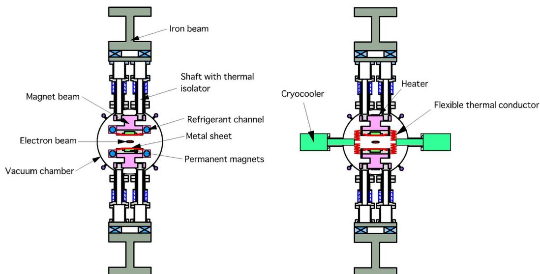
Figure 10.2.1.: Diagram of a typical CPMU structure with two different cooling schemes. Left: refrigerant channels with liquid nitrogen. Right: cryocooler coldheads. Reproduced from [341].
