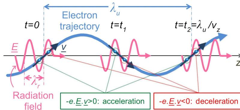
Figure 3.2.: Schematic of the undulator resonance condition. As the electrons traverse one undulator period the radiation propagates forward relative to the electrons by one radiation wavelength, allowing sustained energy transfer. Depending on their longitudinal alignment, electrons either gain or lose energy, which leads to a modulation in the electron beam energy. Figure constructed following the approach of [54]
