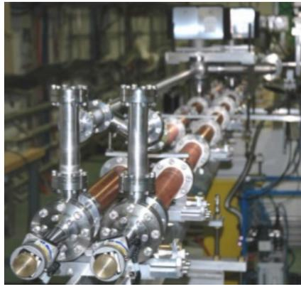
Figure 5.53.: 30 GHz SLED2 pulse-compressor in CTF3.
