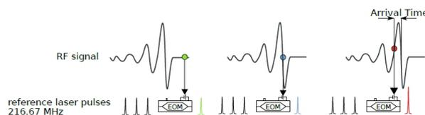
Figure 5.95.: Working principle of the electro-optical unit (EOM).
