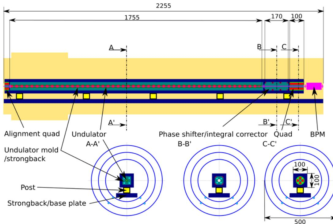
Figure 6.13.: Basic layout of the SCU cryomodule.
