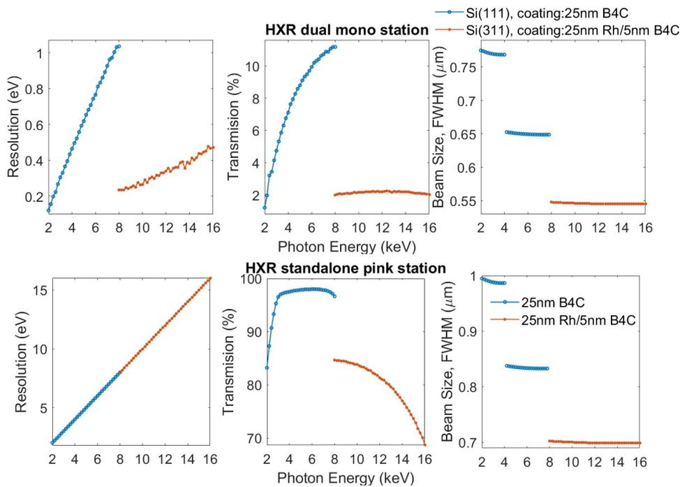
Figure 6.61.: Photon beam parameters on the sample for the  $B_{2d,H,m}$  (top) and  $B_{2s,H,p}$  (bottom) beamlines. The drop in transmission towards the lower photon-energy range, particularly visible for the bottom figure, is due to clipping of the X-ray mirrors at large beam divergence.
