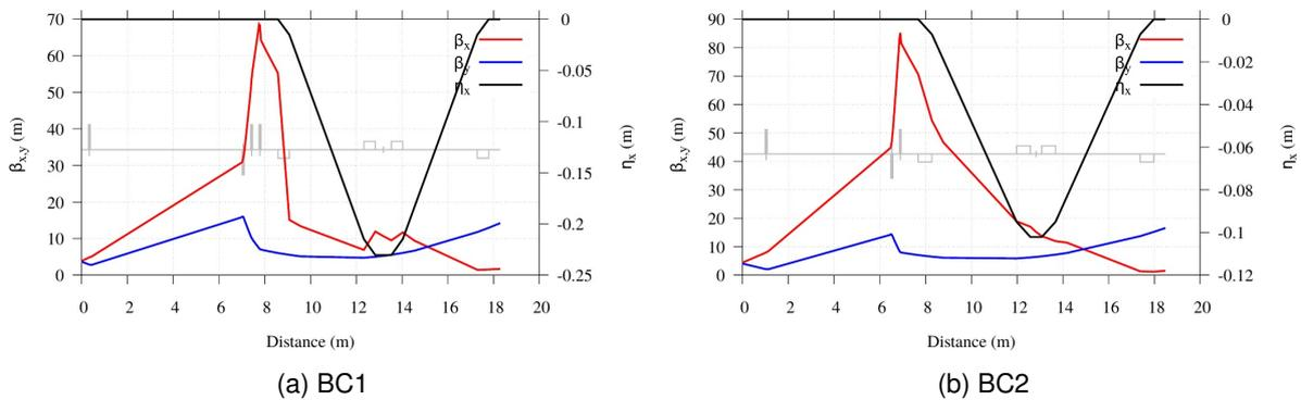
Figure 5.69.: Twiss functions along BC1 and BC2
