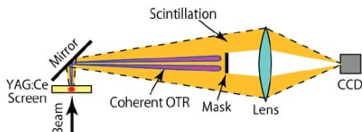
Figure 5.89.: COTR suppression system in use at SACLA [188]
