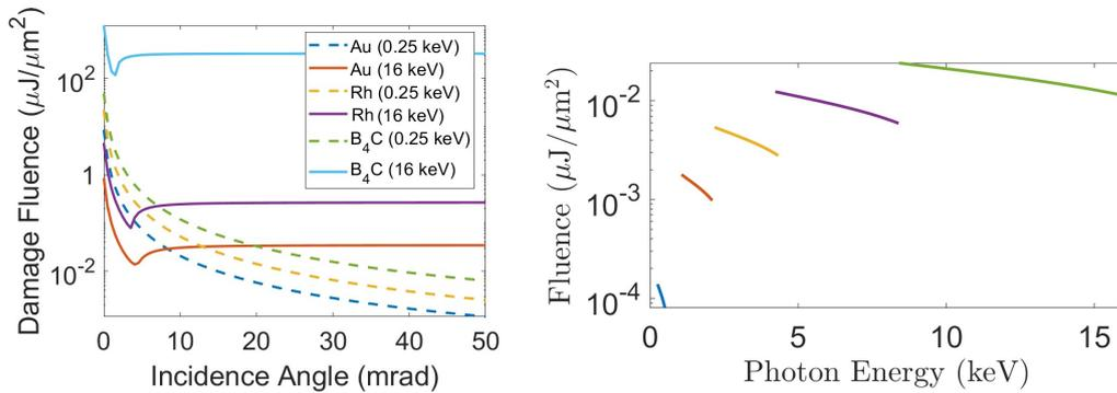
Figure 6.57.: Maximum tolerable fluence vs incidence angle for Au,  $\text{B}_4\text{C}$  and Rh (left plot). The FEL fluence vs photon energy at 50 m away from the virtual source (right plot).
