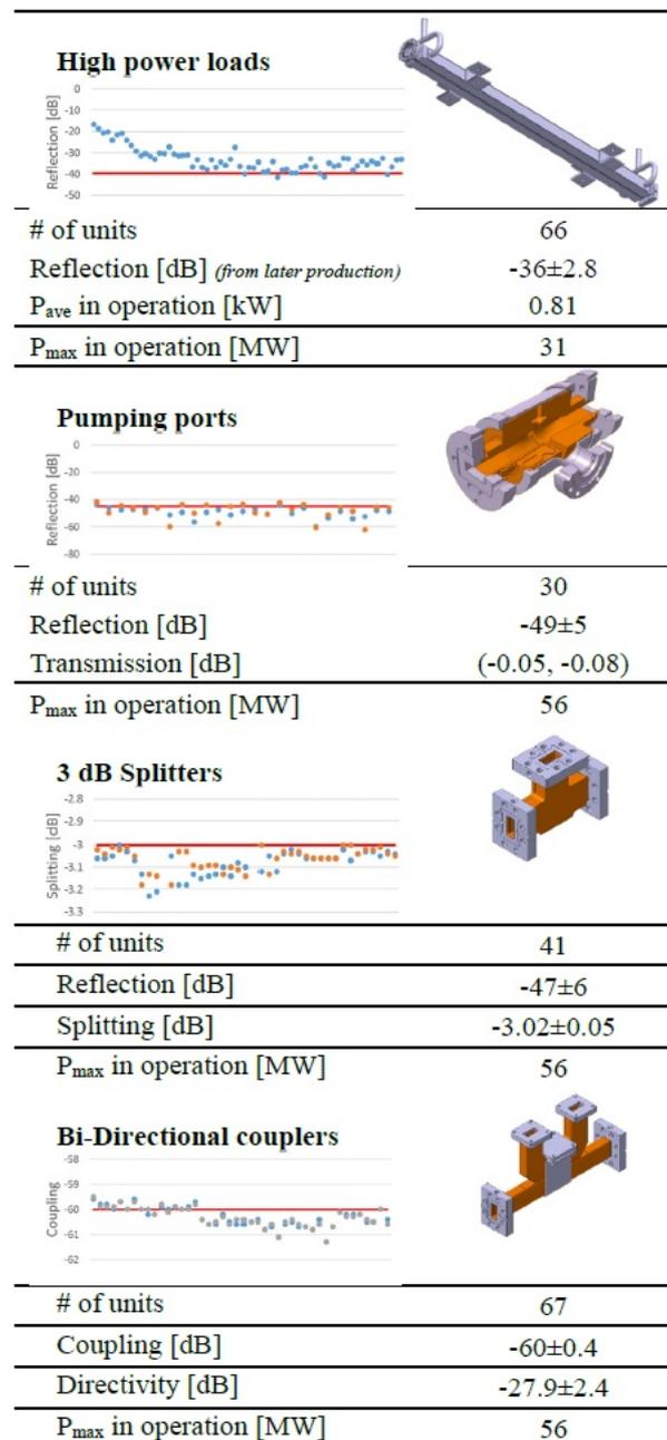
Figure 5.24.: Main parameters of RF components developed by the CLIC group at CERN.
