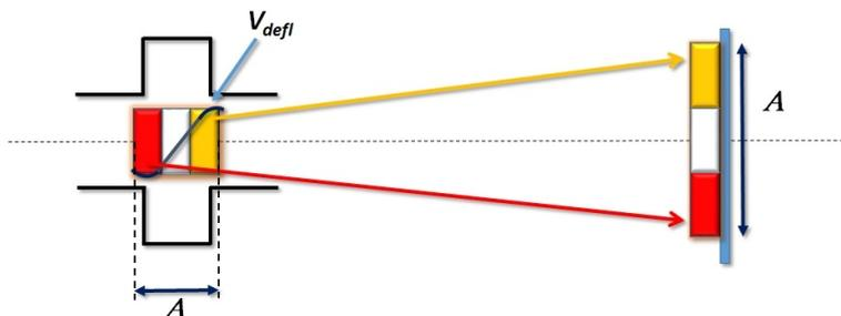
Figure 5.90.: Principle of operation of RF deflector. The longitudinal structure is mapped on the transverse profile because different longitudinal positions experience different transverse kicks.
