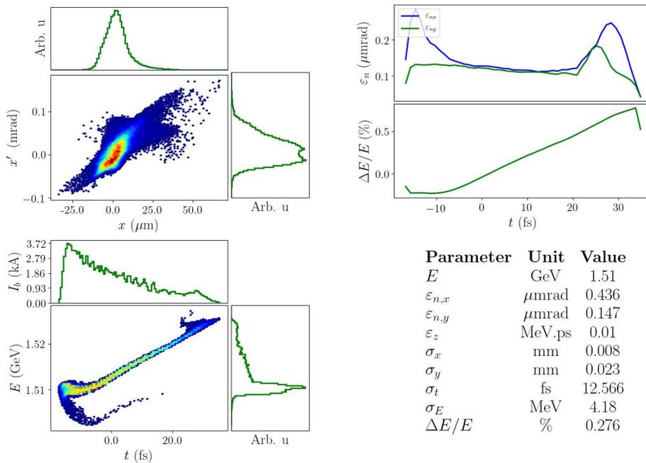
Figure 5.77.: Horizontal (top left) and longitudinal (bottom left) phase spaces with associated histograms representing the projection along the respective axis and sliced emittance/energy spread and beam parameters of the bunch at the exit of low energy spreader.
