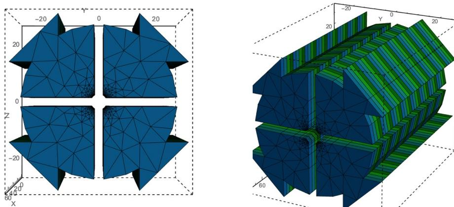
Figure 6.34.: RADIA [251] model of the APPLE-X magnet configuration. The magnetic gap, here, the free diameter depends on in- or out-of vacuum solutions. For a 5 mm inner diameter vacuum chamber, a magnetic diameter of 6.5 mm is required. For in-vacuum undulators this can be reduced to about 5.2 mm. The slit can be minimum 2.5 mm to allow magnetic measurements and support of a vacuum chamber.
