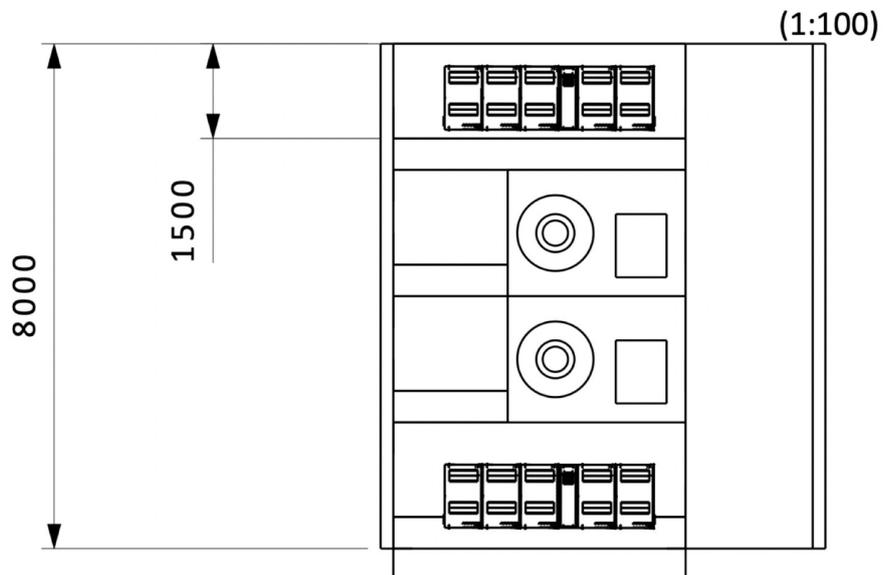
Figure 7.3.2.: Infrastructure Hall - RF cell top view (1:100)
