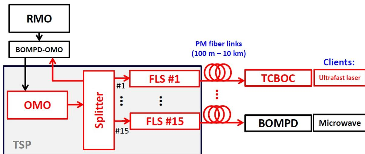
Figure 5.104.: CompactLight optical timing system schematic layout.
