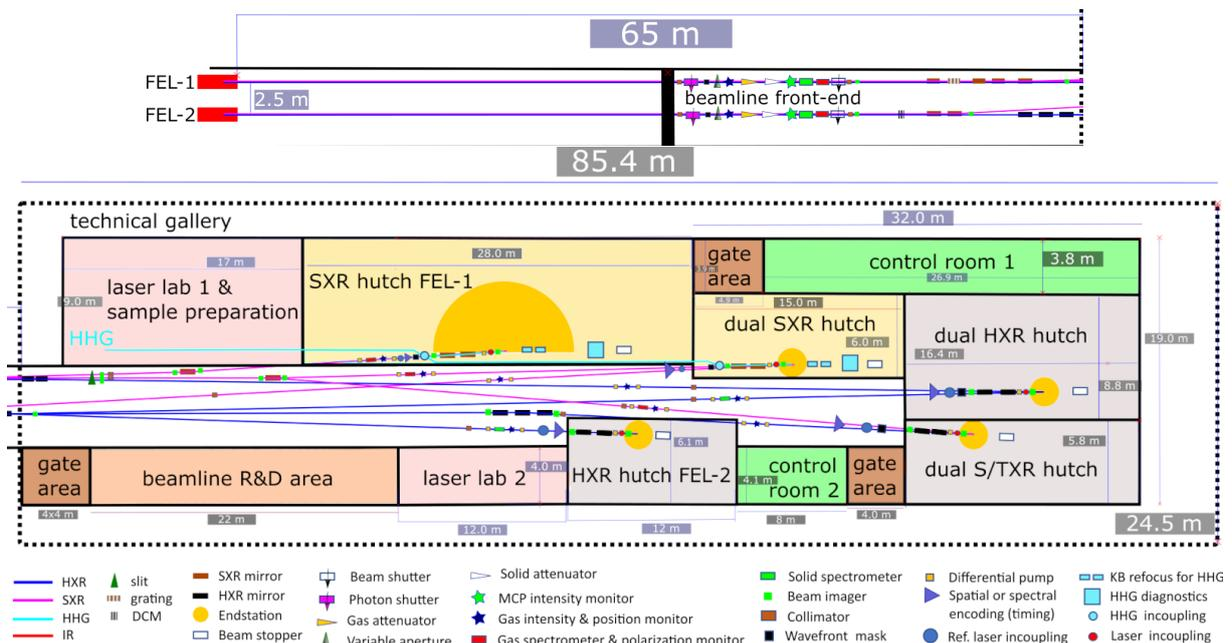
Figure 6.63.: Beamline front-end, experimental area and diagnostics
