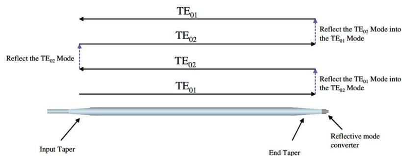
Figure 5.54.: The delay-line of dual-moded SLEDII pulse-compressor.
