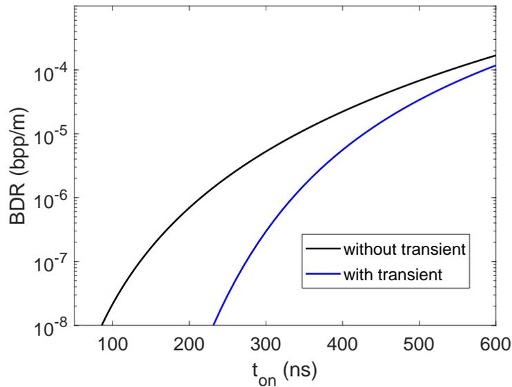
Figure 10.1.8.: BDR in the gun as a function of the RF pulse-length for a constant cathode electric field of 200 MV/m.
