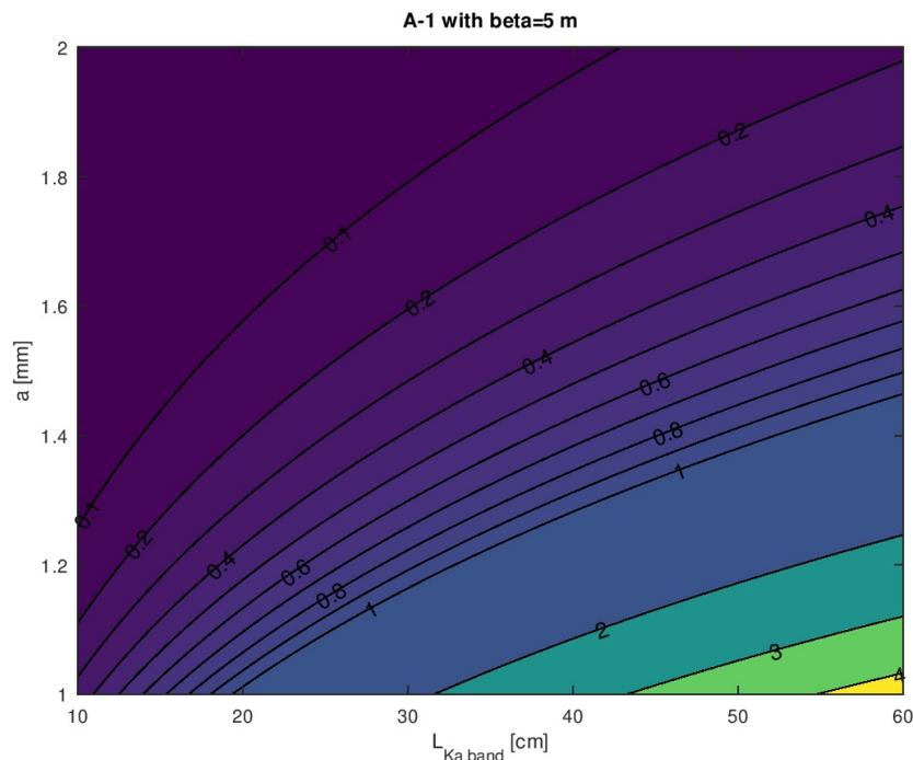
Figure 5.41.: The fraction of the action amplification factor exceeding one under the effects of short-range wakefields in the Ka-band lineariser, as a function of the Ka-band length and of the aperture radius.
