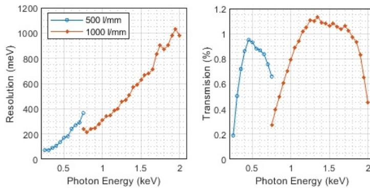
Figure 4.16.: Resolution and Transmission of the SXR self-seeding monochromator.
