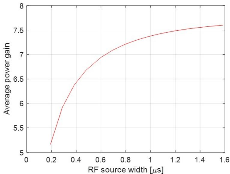
Figure 5.55.: Average power gain from the pulse-compressor as a function of RF power source pulse width.
