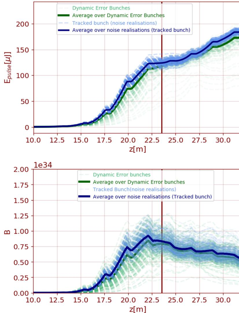
Figure 4.14.: Comparison of 16 keV FEL pulse energy (top) and peak brightness (bottom) for 200 tracked bunches with SASE shot noise and for 200 dynamic error bunches.
