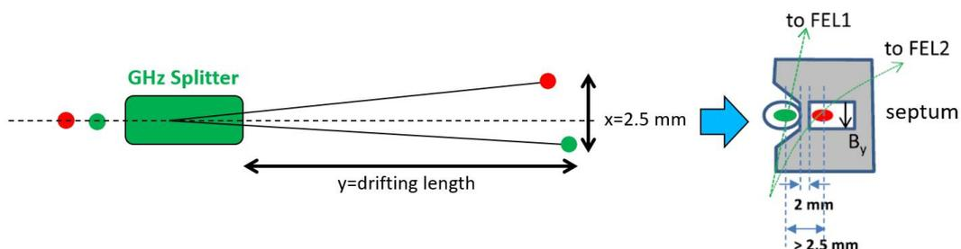
Figure 5.31.: Schematic figure of the S-band splitter system.
