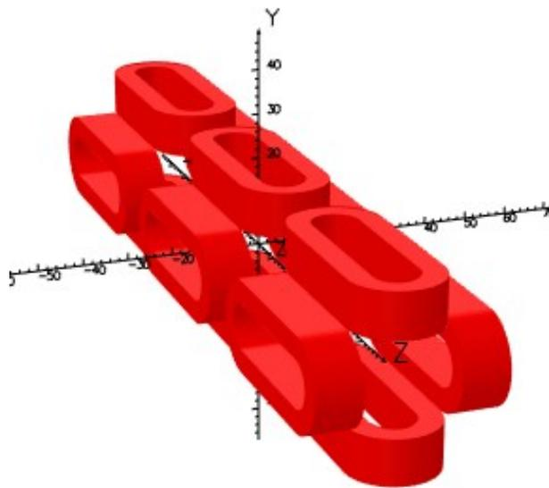
Figure 6.23.: Image of Opera 3D model of phase shifter conceptual magnetic design. The red rings represent superconducting coils.
