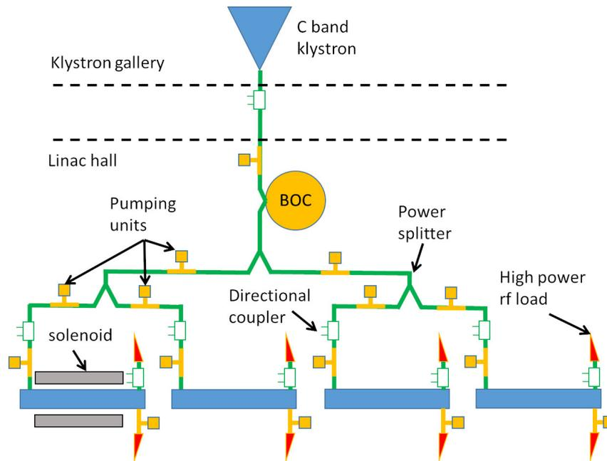
Figure 5.11.: Schematic layout of the C-band booster feeding system
