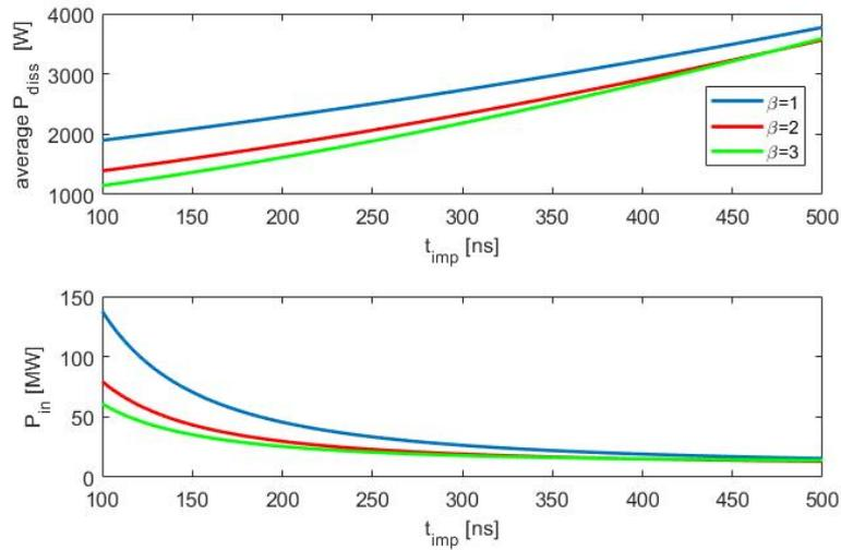
Figure 5.3.: Average dissipated power (upper plot) and required input power (bottom plot) as a function of the rf pulse-length, for three different coupling coefficients.
