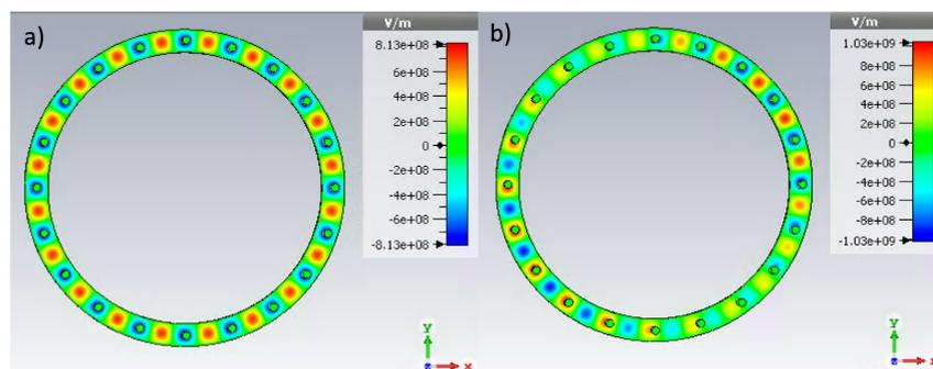
Figure 5.42.: TE<sub>20,1,0</sub> mode (a) and TE<sub>21,1,0</sub> mode (b) in the coaxial cavity with integrated beam tunnels.
