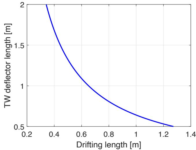
Figure 5.35.: Travelling-wave deflecting structure length versus drifting length. The input power is 31.74 MW.
