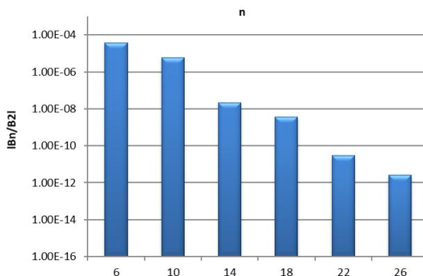
Figure 6.52.: Absolute normalised multipole errors in the 2 mm radius. The quadrupolar component,  $n = 2$ , is not shown.
