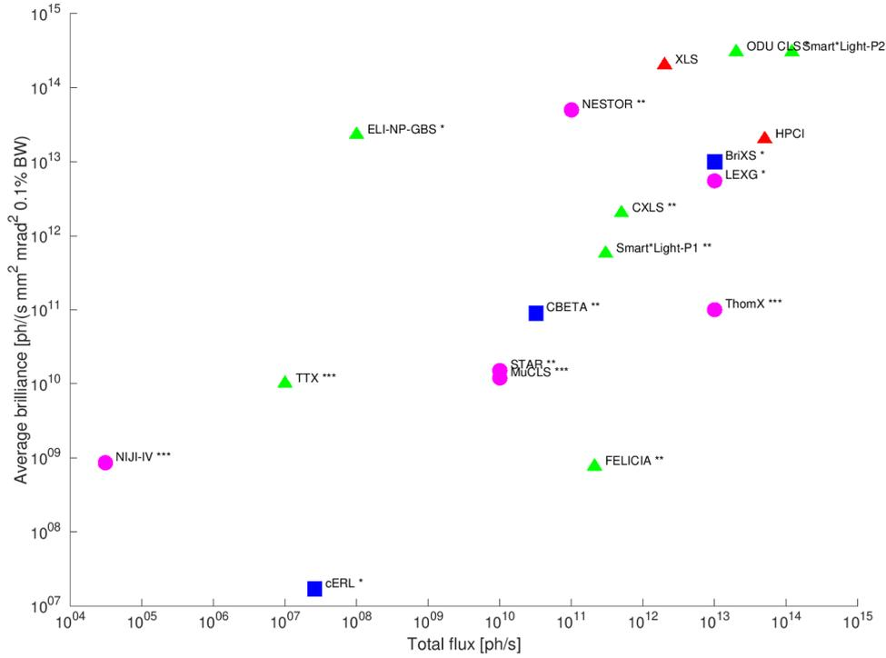
Figure 9.2.2.: Landscape of ICS sources. Circles indicate storage-ring-based sources, triangles indicate linac-based sources, squares energy-recovery-linac-based sources. Stars indicate: \*, design study; \*\*, under commissioning; \*\*\*, existing.
