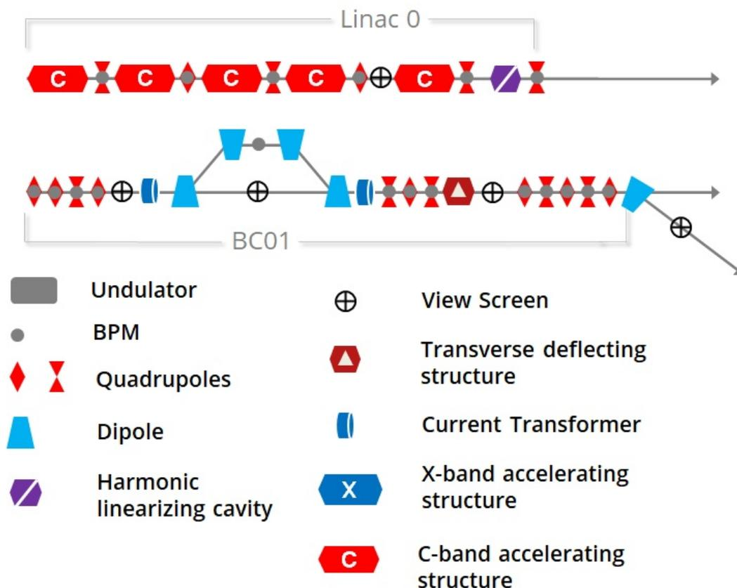
Figure 5.98.: Schematic definition of the diagnostics in the region surrounding the bunch compressor 01.
