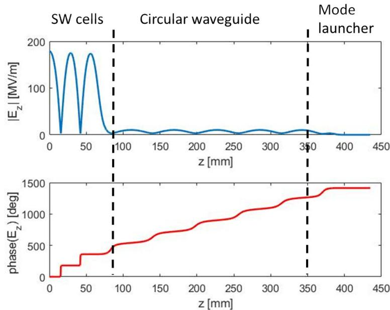
Figure 5.5.: Magnitude and phase of the longitudinal accelerating field on axis.
