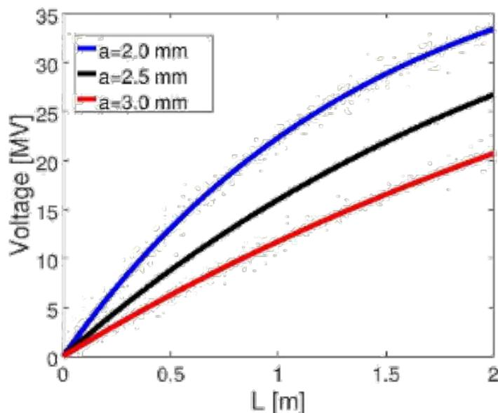
Figure 5.40.: Analytical estimate of the required voltage as a function of the Ka-band length, for different iris aperture radii.
