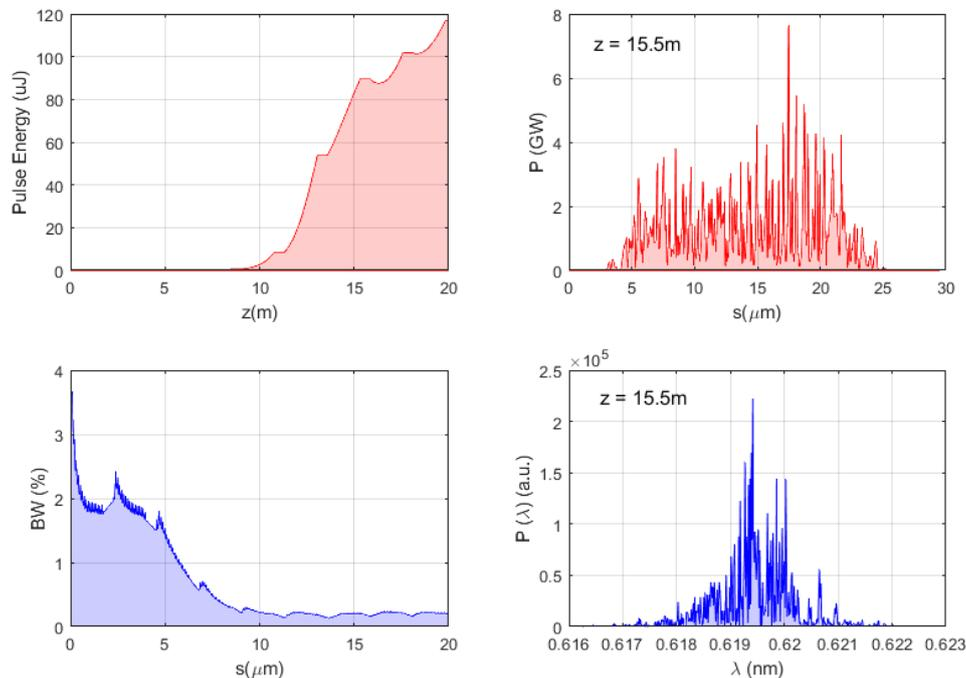
Figure 9.1.4.: FEL simulation results of the SXR FEL performance, showing (top left) pulse energy vs distance through the undulator  $z$ , (top right) power profile of output pulse at saturation, occurring at  $z = 15.5$  m, (bottom left) rms bandwidth vs  $z$ , and (bottom right) pulse spectrum at saturation.
