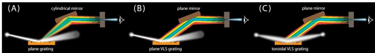
Figure 6.59.: Types and mount of a grating-based monochromator.
